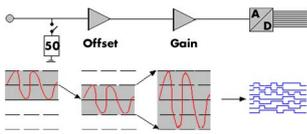
The analog inputs can be adapted to real world signals using a wide variety of settings that are individual for each channel. By using software commands the input termination can be changed between 50 Ohm and 1 MOhm, one can select a matching input range and the signal offset can be compensated for.
