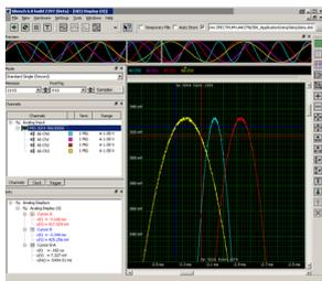
The digitizerNETBOX and generatorNETBOX can be used with Spectrum's powerful software SBench 6 – a Professional license for the software is already installed in the box. SBench 6 supports all of the standard features of the instrument. It has a variety of display windows as well as analysis, export and documentation functions.
